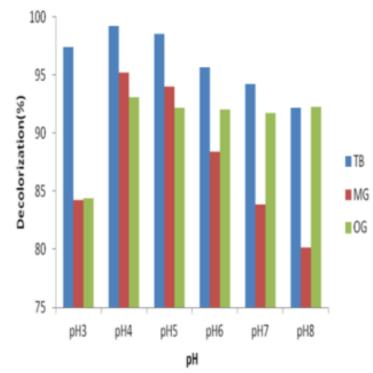
Figure 1: Effect of pH towards decolorization of three prototypical dyes by oxidizing agent (Sodium hypochlorite)
